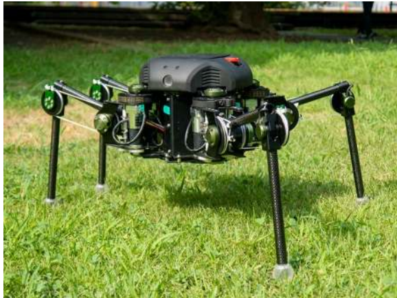
Fig. 2 Sprawling-type quadruped robot TITAN-XIII
