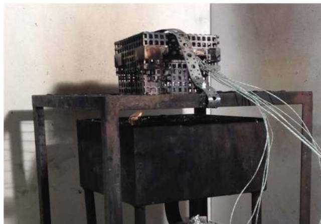
Figure 8. Photo of test type A, showing the 5-cell-pack inside a steel-net-box placed on the wire gratings. The sand bed for the propane burner is underneath the wire grating, a pilot flame (seen in front left corner of the burner) is used to ignite the propane gas.
